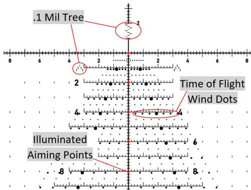
The illuminated TREMOR5 features illuminated aiming dots at the center, on the primary vertical stadia every 2 mil-radian below center, and at 2 mil-radian of windage left and right on the 10 mil-radian horizontal stadia.
