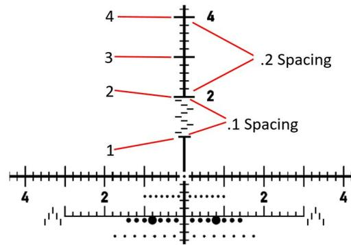
The TREMOR5 incorporates milling chevrons for both height and width range estimating. With the chevron shape you're able to very precisely estimate the range to your target. The below example demonstrates how to use the Refined Milling Chevrons with the Horus Ballistics App:
